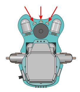
The light sensors produce a small electric voltage that Wink's brain can measure and turn into a number. This number represents how much light is falling on each of the sensors. The sensors can provide a reading between 0 and 1024. It should be noted that the level may not reach all the way down to 0, and it will likely not reach all the way to 1024, but it will get close. This is okay and normal.
